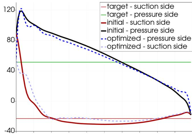
Figure 4: Pressure distribution over the blade profile.
