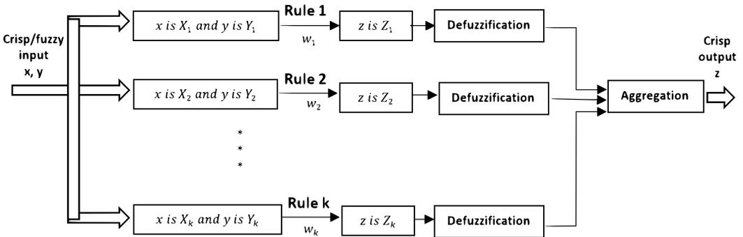
Fig. 5. FIS with rule-based defuzzification (FIS-RBD).
